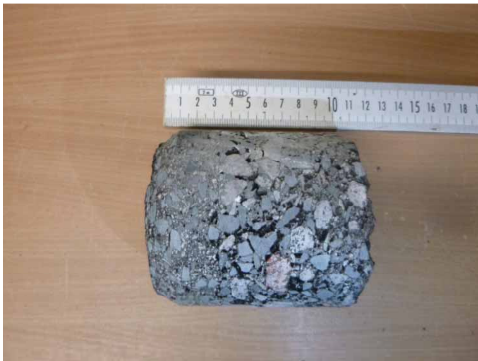
Foto 2: Asphaltbohrkern RKB 18 (AP 1)
