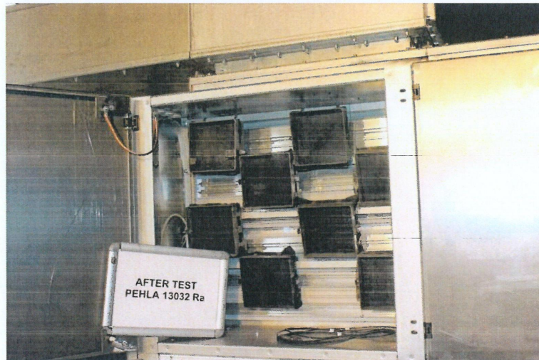
Photo No. 12 After test PEHLA 13032Ra / 03 Additional indicators within low-voltage compartment
