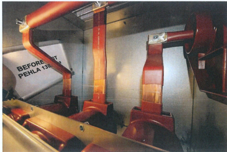
Photo No. 01 Before test PEHLA 13031Ra / 06 Initiation wire across tee-off busbars
