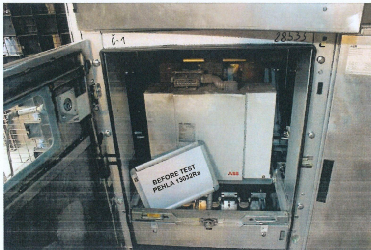
Photo No. 02 Before test PEHLA 13032Ra / 03 Test object, front view with doors of left-hand side panel opened.
